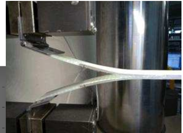
Interlaminar Fracture Toughness Energy (mode I), G_{1c} from DCB specimen (ISO 15024)
