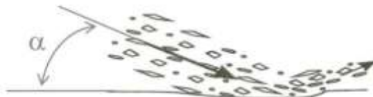
Fig. 2: Schematic illustration of impingement angle \alpha in SJE testing.
